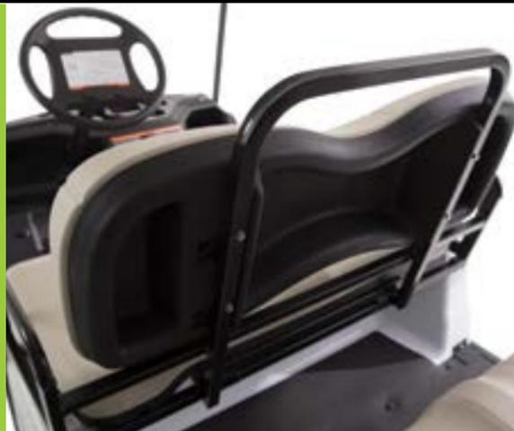
Our rugged, powder-coated steel handle provides additional comfort and safety for rear seat passengers.
